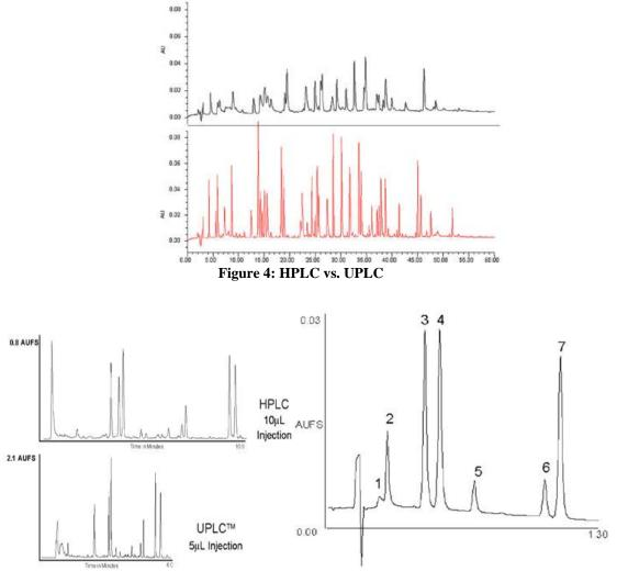
Figure 5: Comparison of Natural Product Extraction with UPLC and HPLC
