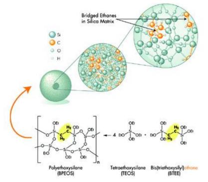
Figure 1: Synthesis and Chemistry of ACQUITY 1.7µm particles for UPLC
