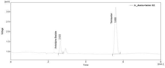
Figure 1: A typical chromatogram of amlodipine and telmisartan
