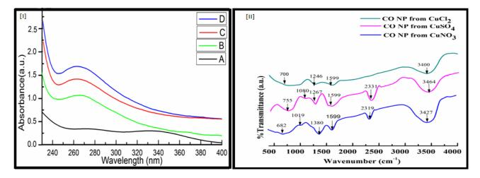
Figure 1: (I) UV-Vis absorbance- A. Raw plant electrolyte; B.CONP derived from CuNO<sub>3</sub>; C. CONP derived from CuSO<sub>4</sub>; D. CONP derived from CuCl<sub>2</sub>. (II)FTIR Spectra of CONP
