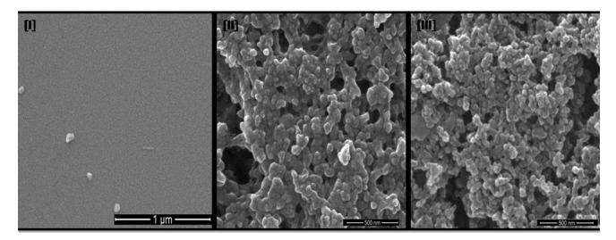
Figure 2: SEM images of CONP :(I)CONP derived from  $CuCl_{2,}$ , (II)CONP derived from  $CuSO_{4,}$  (III) CONP derived from  $CuNO_{3}$
