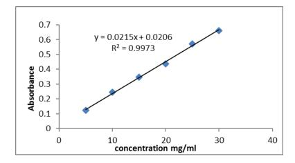
Figure No.2: Standard calibration curve of Lornoxicam in 0.1 N NaOH
