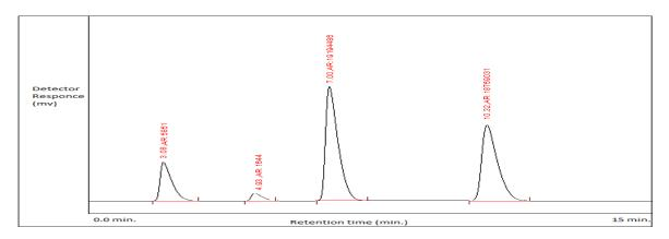
Figure 4: Chromatogram of alkaline hydrolysis 1M NaOH 1 h. reflux at 80°C
