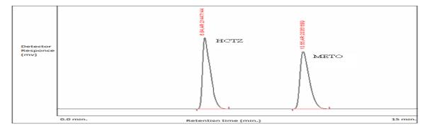
Figure 2: RP-HPLC chromatogram of HCTZ and METO at 222 nm
