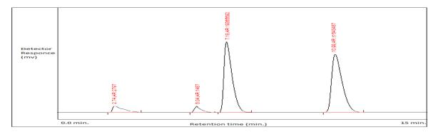
Figure 3: Chromatogram of acid hydrolysis 1M HCl 1 h. reflux at 80°C
