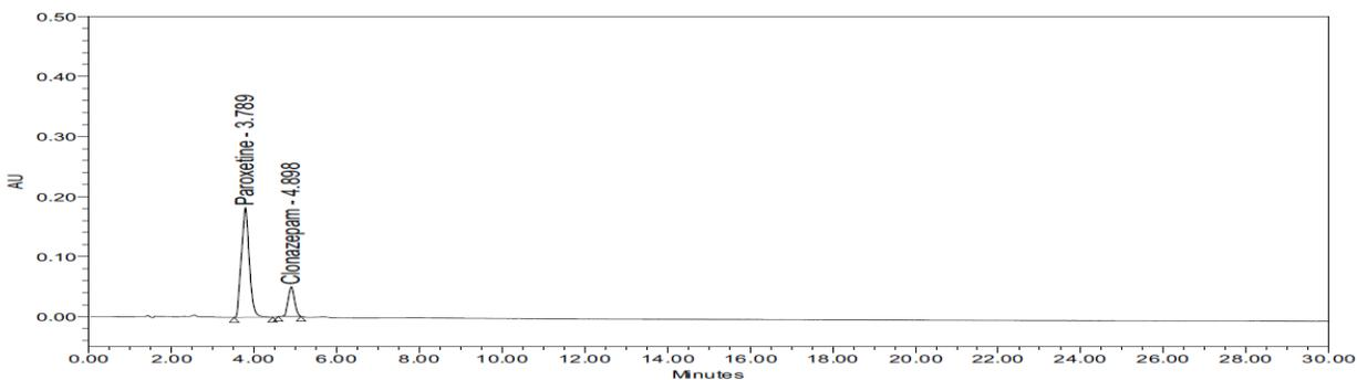
**Figure 8:** Neutral degradation degradation chromatogram of Paroxetine and Clonazepam
