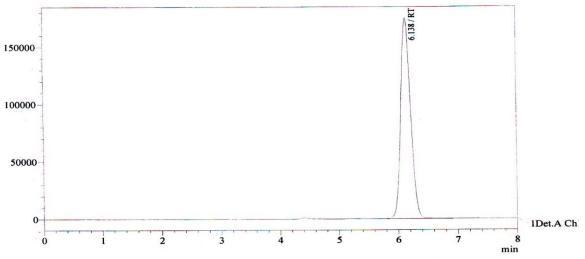
Fig. 2: Chromatogram of Daclatasvir Di-hydrochloride ( $R_T = 6.138$  min)
