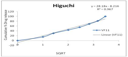
Fig.5. Higuchi release mechanism of VF-11 formulation
