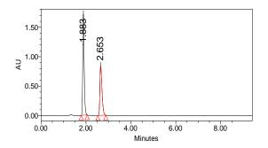
Fig. 4: Chromatogram of sample preparation
