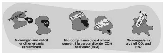
Figure 2: Schematic Diagram of Aerobic Biodegradation in Soil.
