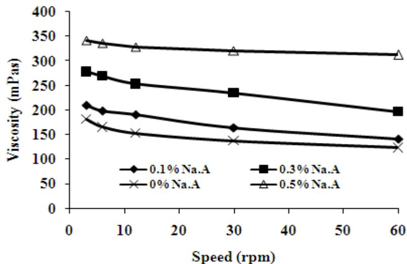
Figure 2: Effect on rpm on viscosity of the formulations.
