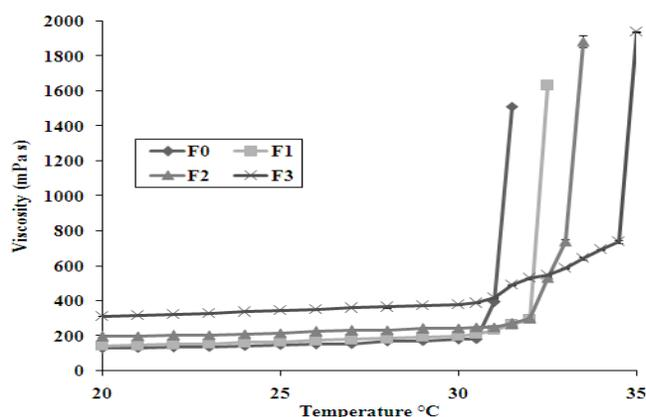
**Figure 1:** Effect of temperature on viscosity of various Pluronic F127 gels with varying concentration of Sodium alginate (0.1% to 0.5%) measured at 60 rpm. Values are expressed as mean ± SD (n=3)
