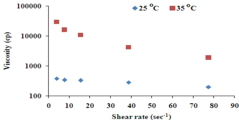
Figure 3: Effect of shear rate on viscosity of F2 at 25°C and 35°C
