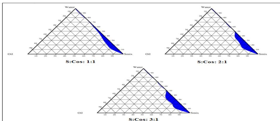
**Figure 1:** Pseudoternary phase diagrams of microemulsion containing sesame oil
