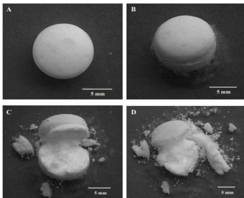
Fig. 3: Sequential presentation of swelling followed by rupture of the outer membrane leaving inner active layer exposed to dissolution media. [42]
