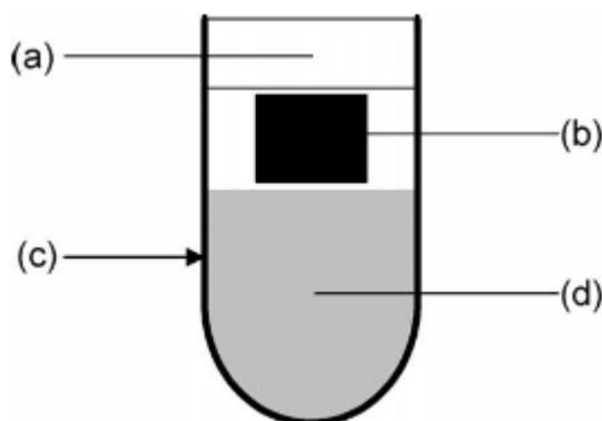
Fig. 1: Pictorial presentation of a osmotic controlled chronomodulated device. (a) erodible or insoluble cup, (b) core of active drug substance, (c) semipermeable outer shell, (d) swellable or osmotic pressure generating agent. <sup>[33]</sup>
