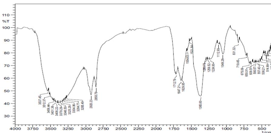
Figure 4. FTIR spectrum of ethanol extract of *Hypnea musciformis*
