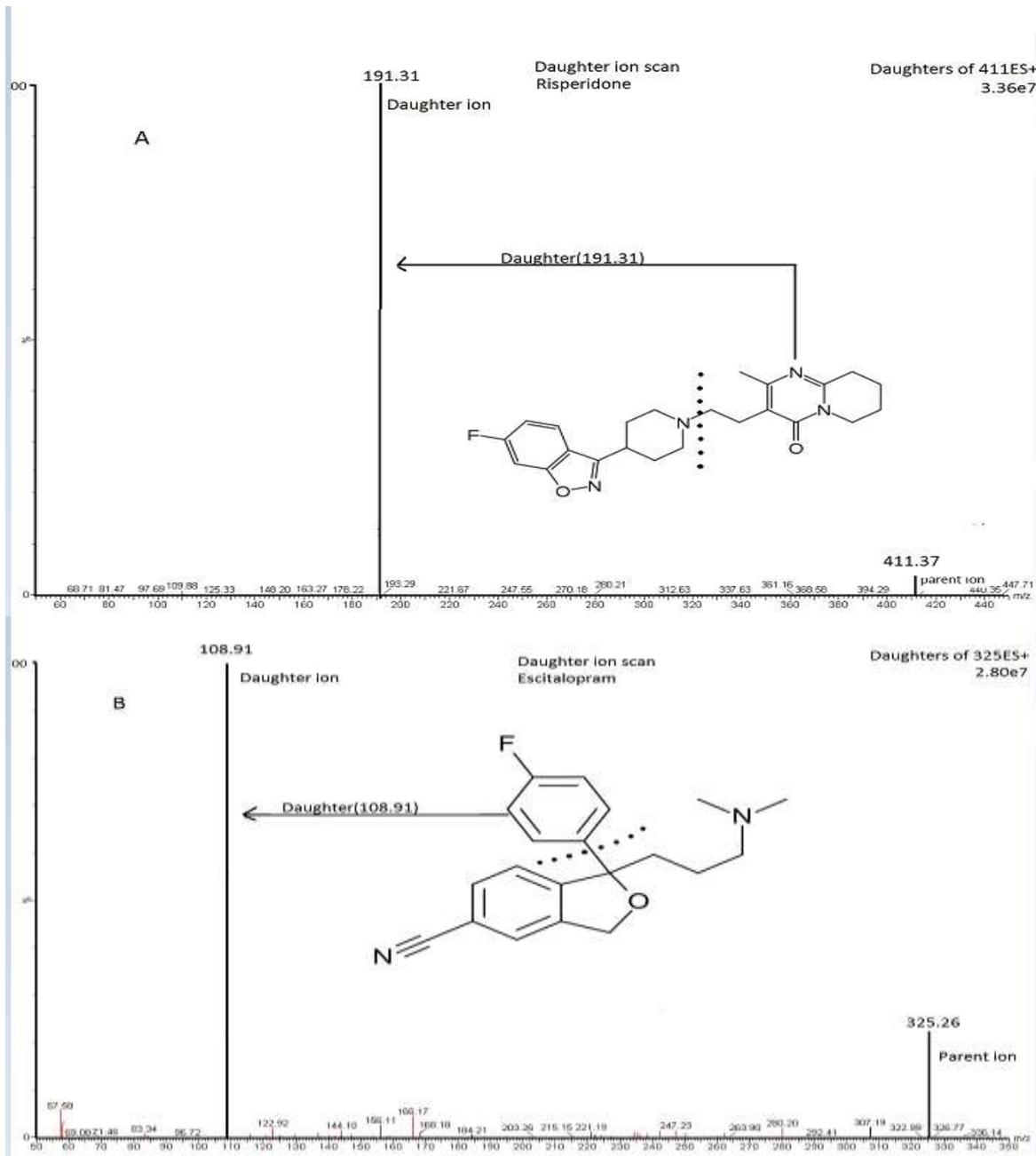
Figure 2. The production mass spectra of risperidone and escitalopram
