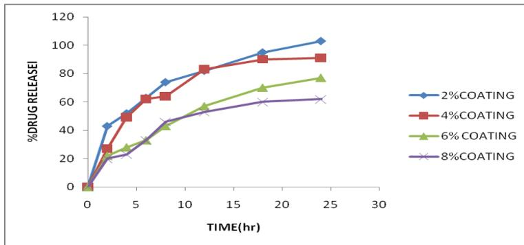
**FIGURE 3 :** Effect of Coating weight gain
