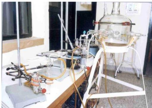
**Fig. 5:** Inhalation assembly used for exposure of C-Compressed air only, F-furfural alone (95ppm), K-Kerosene alone (426-1054ppm), K+F-furfural and kerosene vapors (95ppm) and (426-1054ppm) respectively
